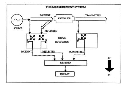
Figure 1: Microwave measurement system
